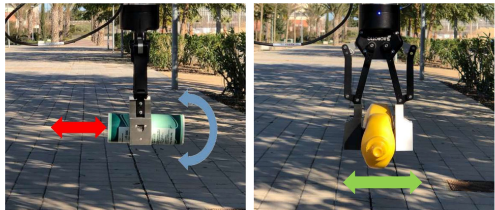
Fig. 15 Translational (red and green) and rotational (blue) perturbations produced by a human operator. These movements include all perturbations that the object could undergo during the manipulation task
